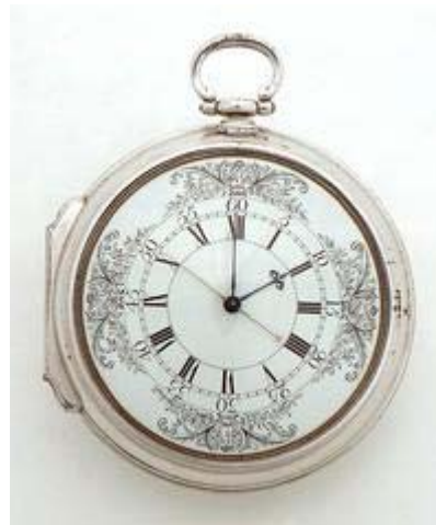
K1 Marine Chronometer(Kendall's copy of Harrison's H4) Repro ID D9661 © NMM London
